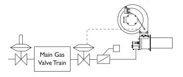
1. Drive the gas control valve to low fire.
